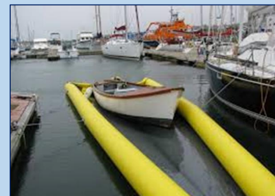
Left: Collecting and filtering water samples for eDNA analysis. Right: a prototype in-water quarantine berth.
